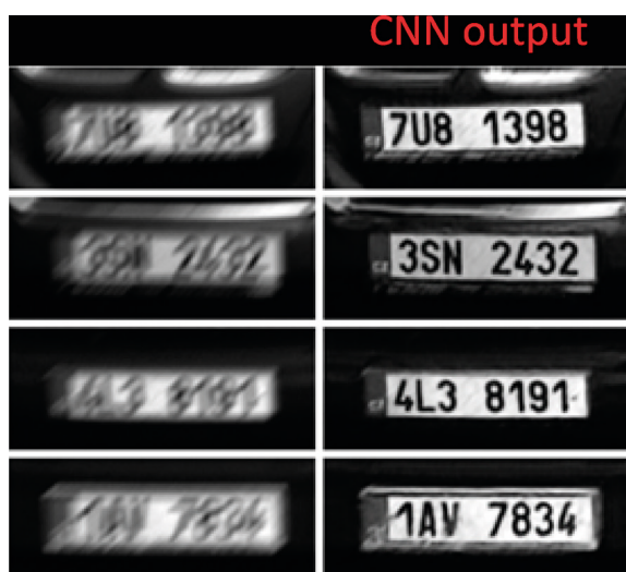
Figure 5. Result of license plate deblurring on images from real-life traffic surveillance system
